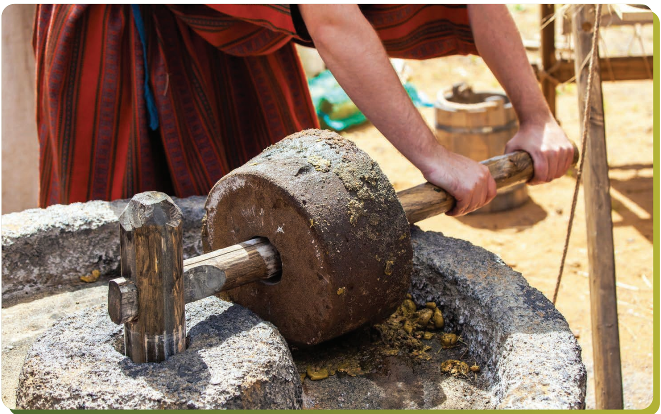
Figure 1 : One of Oil presses used in ancient times for olive oil extraction
