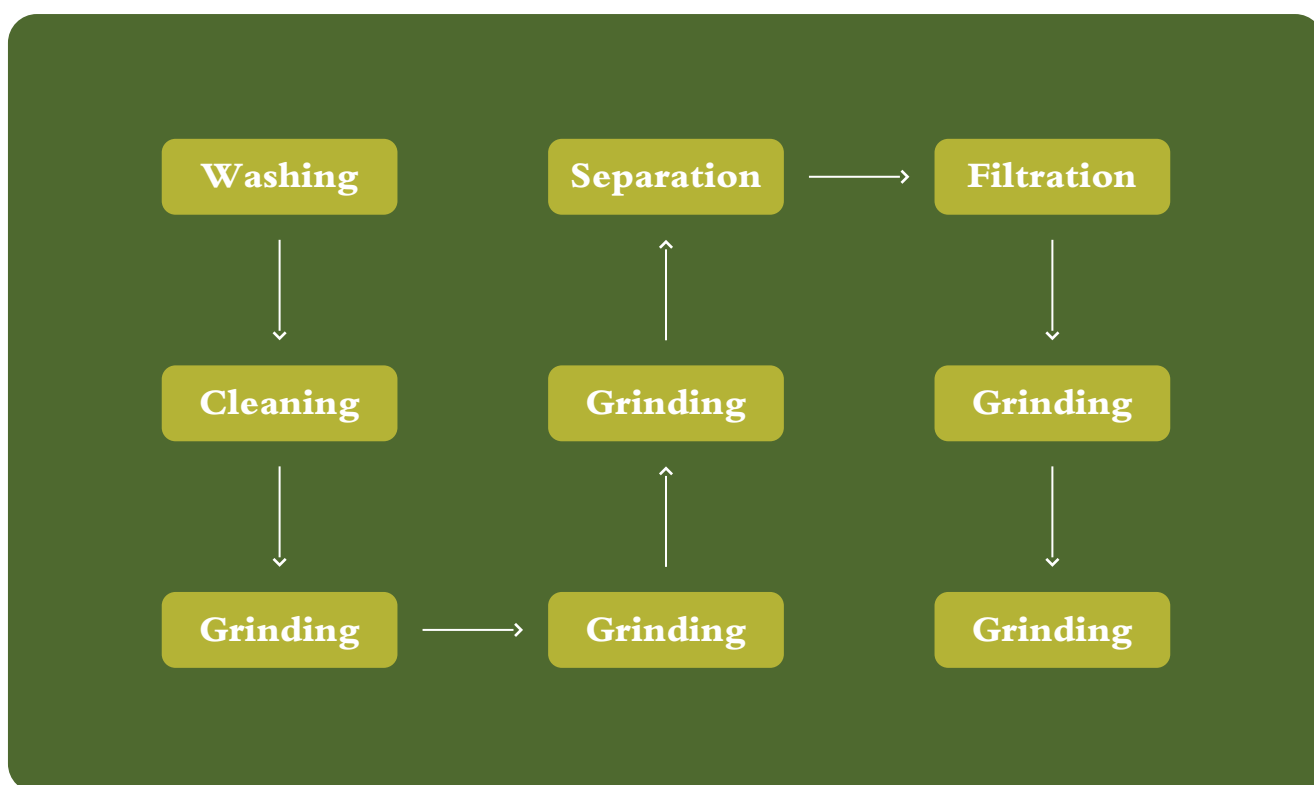
Figure 6: Extraction Process of Olive Oil
